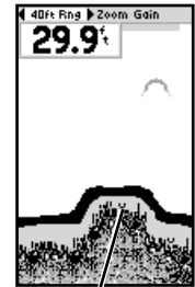
Structure is soft, probably a mud pile
